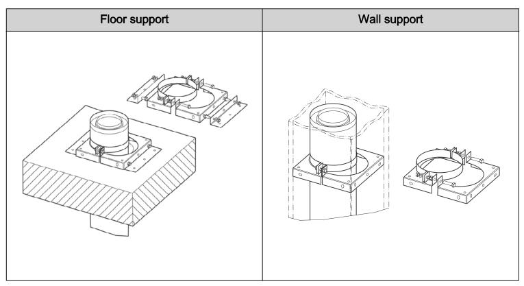
Install a concentric flue system as described in this section.
